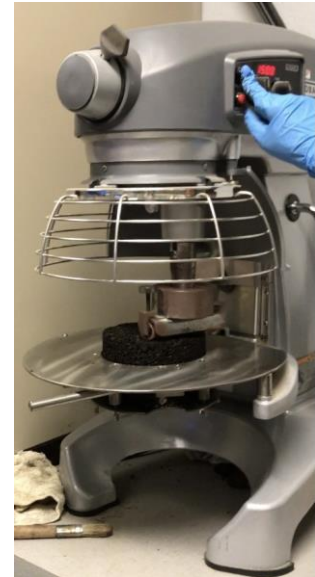
Figure 16. Hobart mixer for raveling test
